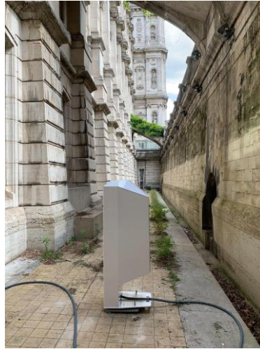
Figure 2. Placement of an ALC in an urban setting below ground level. Such a placement allows to discard the first measurement levels from the analysis without losing information near the surface. Given measurements in the first levels have a relatively high uncertainty for many ALC, this can improve the detection of shallow layer heights. Photo: M. Haeffelin.
