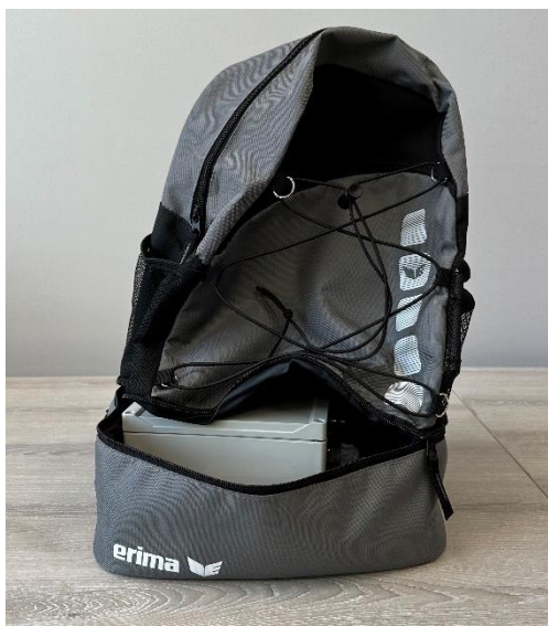
Figure 3. Mobile OPC-N3 setup. The sensors were put in the shoe compartment, leaving the rest of the backpack space free, and were powered by a power bank. There was enough space for additional sensors if needed. The total added weight was less than 1 kg.
