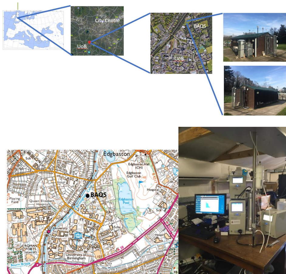
Figure 2.2.1. BAQS Birmingham Air Quality Supersite (urban background) in Birmingham, UK. Upper panel: Overview of the positioning of the site. Lower left panel: location of BAQS within the University grounds. Lower right panel: Photograph of the upgraded MPSS and CEN system to ACTRIS standards, now scanning from 10-800 nm.
