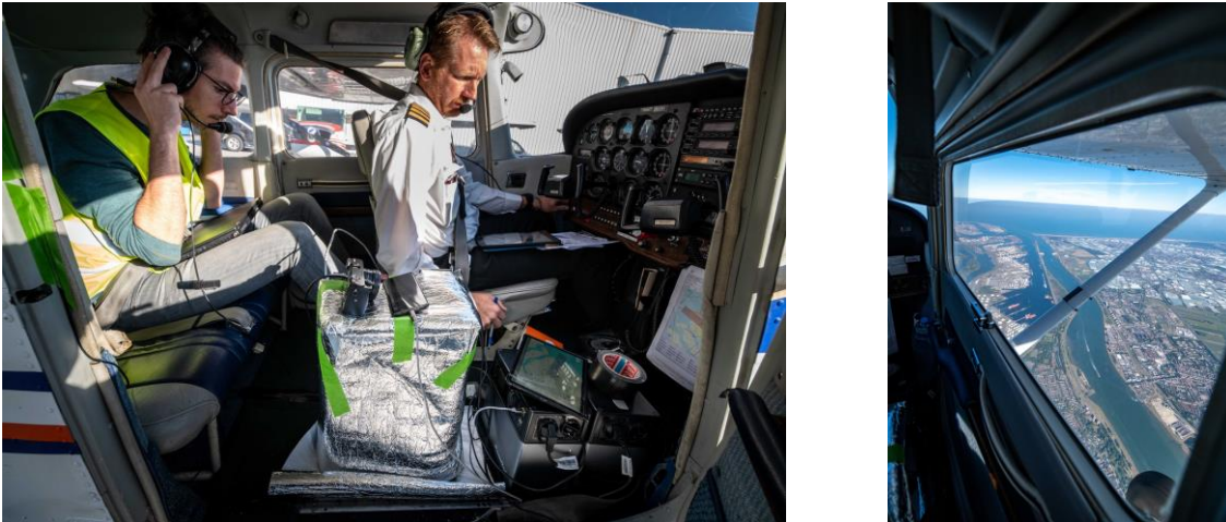
Figure 2.1.9. The Spectrolite instrument mounted in a Cessna Skyhawk single engine aircraft (left) flying over the city and harbor/industrial area (right) to map NO 2 vertical column densities (VCD) (See Figure 2.2.10).
