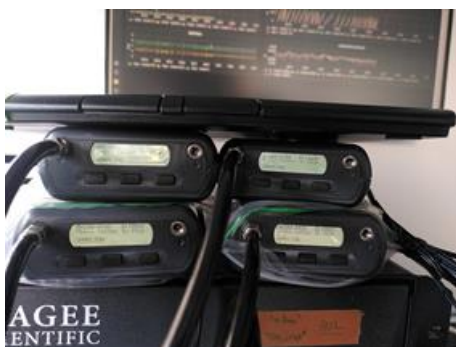
Figure 2.3.7. Intercomparing among the micro-aethalometers and the reference instrument AE-33 were carried out before, during and after the bike field campaign.
