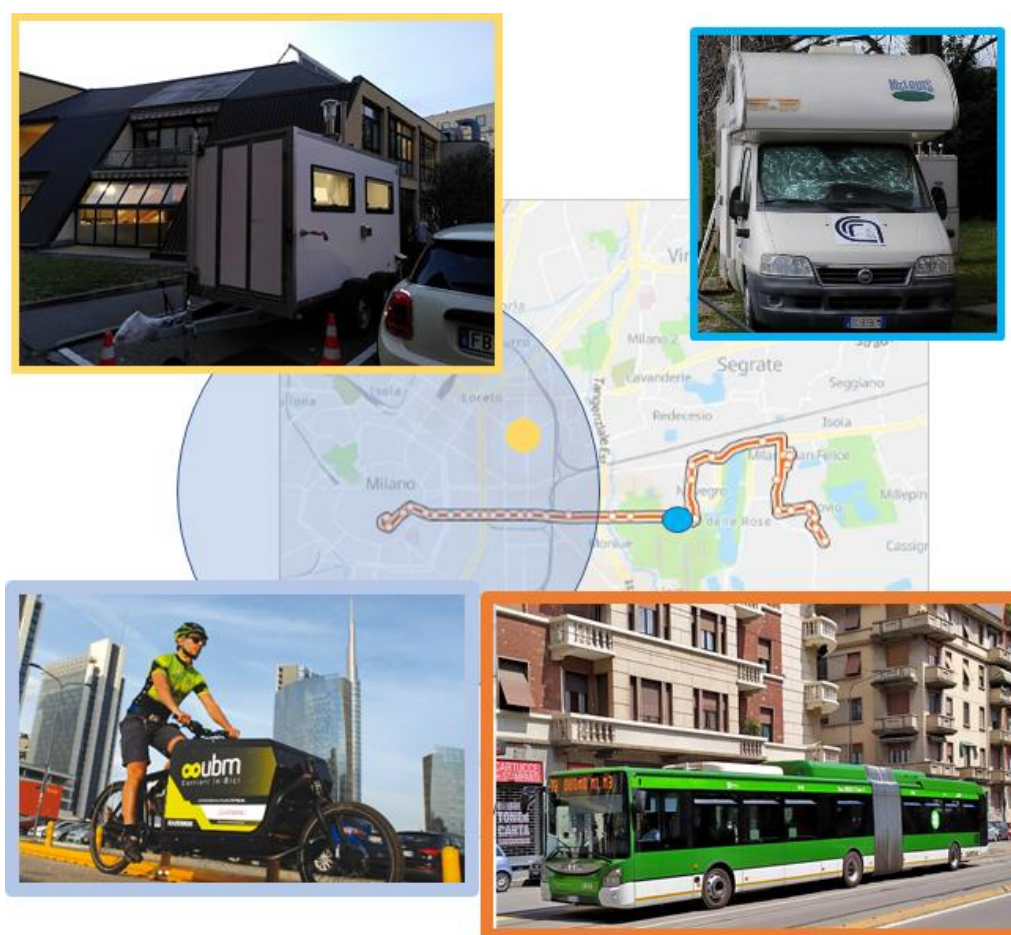
Figure 2.3.3. Area where the fixed and mobile measurements occurred during the 2023 field campaign were located. The orange line represents the route of line 73 bus (targeted mobile measurements on a planned fixed route), while the blue area represents the area where the opportunist measurements are performed, by using existing delivery cyclists' daily routines.
