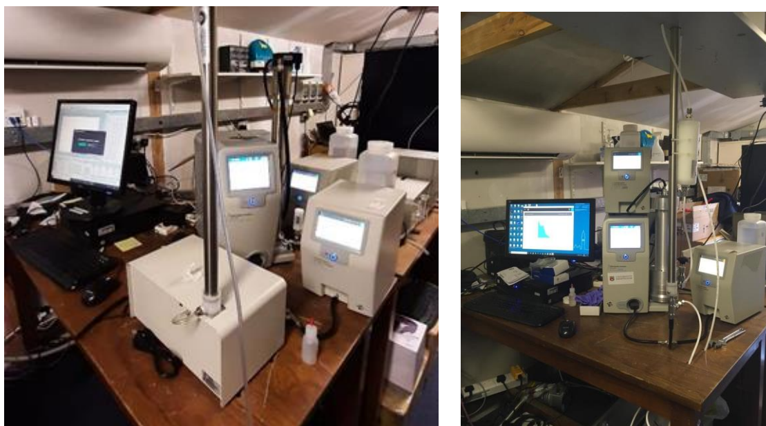
Figure 3. Left panel: A photograph of the original MPSS system at BAQS. Right panel: A photograph of the upgraded MPSS and CEN system to ACTRIS standards, now scanning from 10-800 nm. More recently adapted to include a 4 ways aerosol splitter, not shown in photograph.
