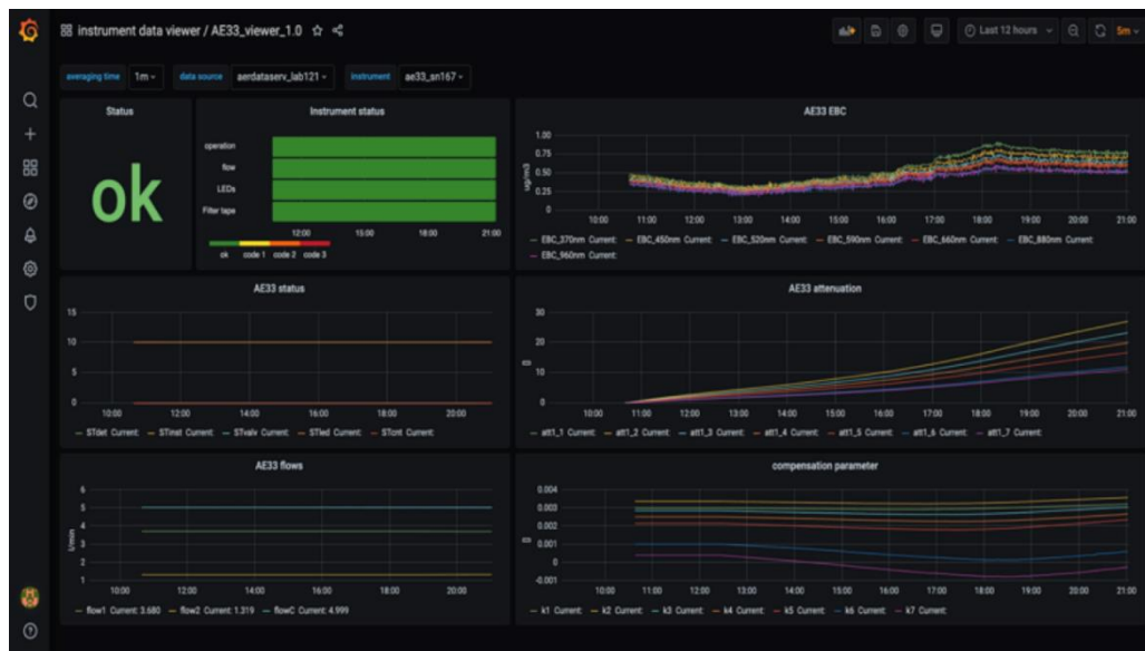
Figure 7: Screenshot of the real-time visualisation with access to data archive (local database).
